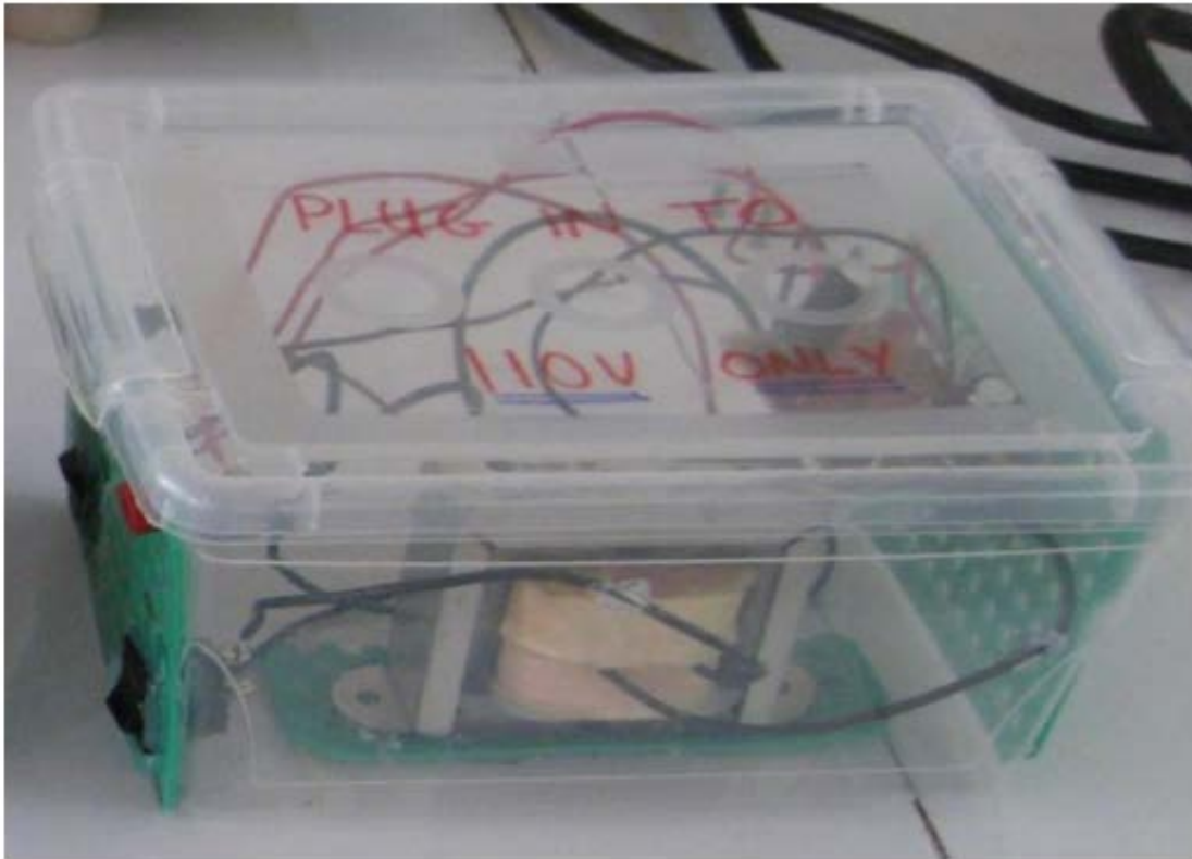
Figure 5: SBPSU with secured cover and warning label indicating only 110V AC input
