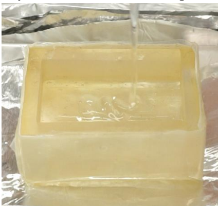
Figure 2: The figure shows a mould being filled with PDMS.
