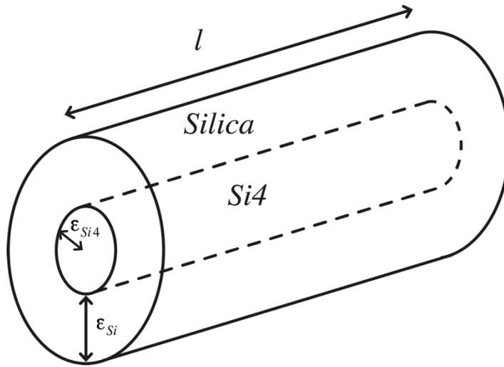
Schematic of the model: silica forms a cylindrical layer that coats the linear cylinder of the Si4 protein
