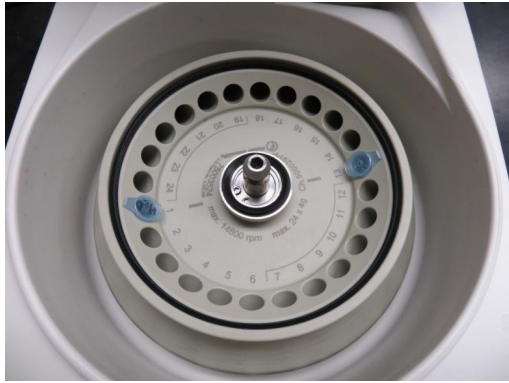
Figure 15 – A balanced rotor in which each tube is opposite another tube with the same volume .
